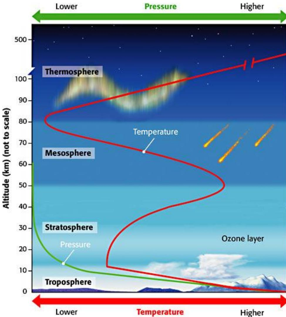
**Figure 3** The layers of the atmosphere are defined by changes in temperature.
