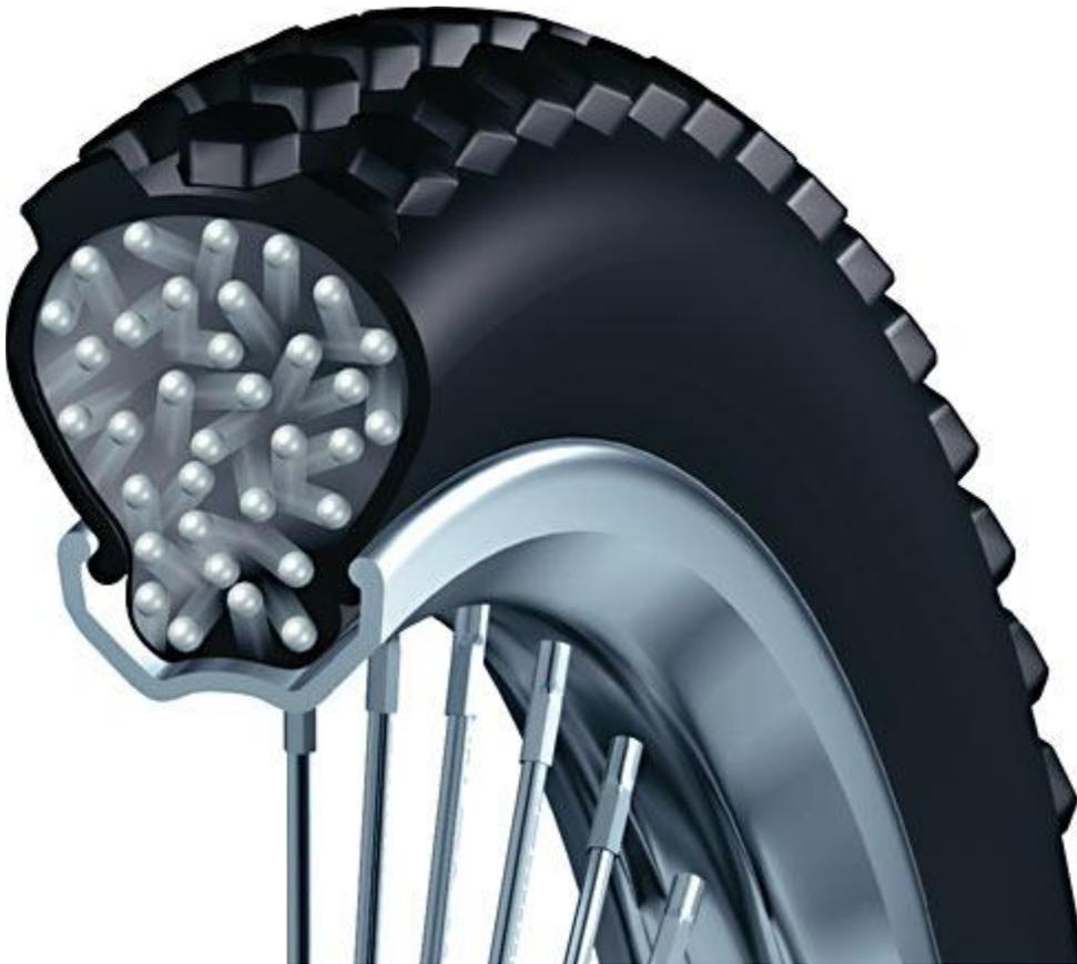
**Figure 1** The force of the air particles hitting the inner surface of the tire creates pressure, which keeps the tire inflated.
