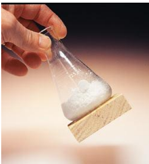
Figure 6 The reaction in the flask absorbs energy and causes water between the bottom of the flask and the wood to freeze.
