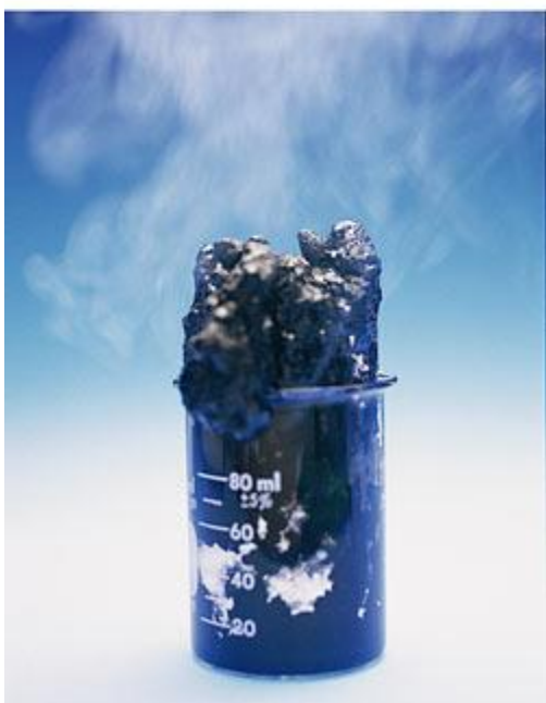
Figure 3 The top photo shows table sugar, a white solid, being mixed with sulfuric acid, a clear liquid. These two starting substances react to form new substances that are very different from the sulfuric acid or sugar. What are some of the properties of the new substances?
