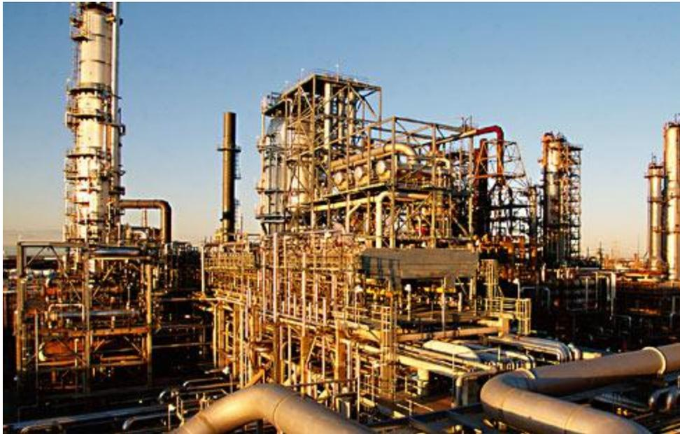
**Figure 2** This refinery uses a process called distillation to separate petroleum into various types of petroleum products.
