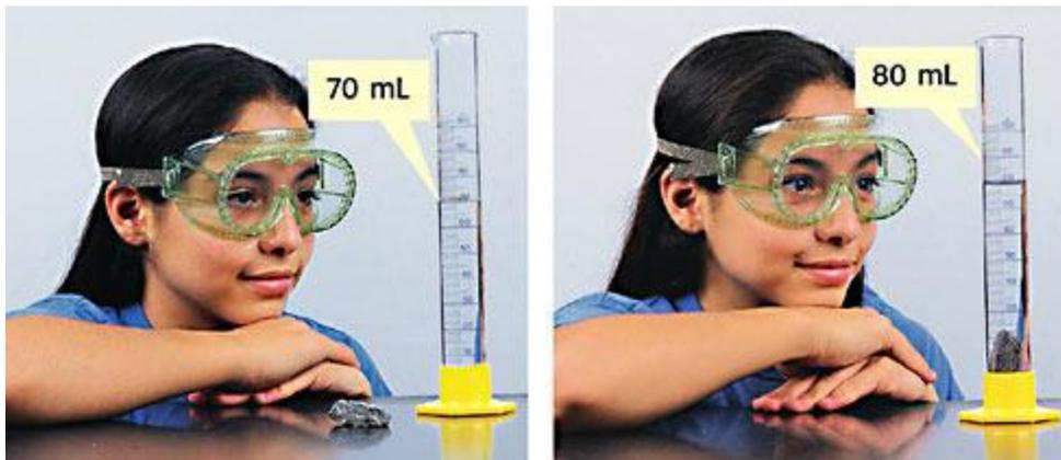
**Figure 5** Adding the rock changes the water level from 70 mL to 80 mL. So, the rock displaces 10 mL of water. Because  $1 \text{ mL} = 1 \text{ cm}^3$ , the volume of the rock is  $10 \text{ cm}^3$ .
