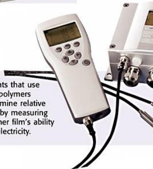
Instruments that use thin-film polymers can determine relative humidity by measuring the polymer film's ability to store electricity.
