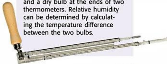
A psychrometer has a wet bulb and a dry bulb at the ends of two thermometers. Relative humidity can be determined by calculating the temperature difference between the two bulbs.
