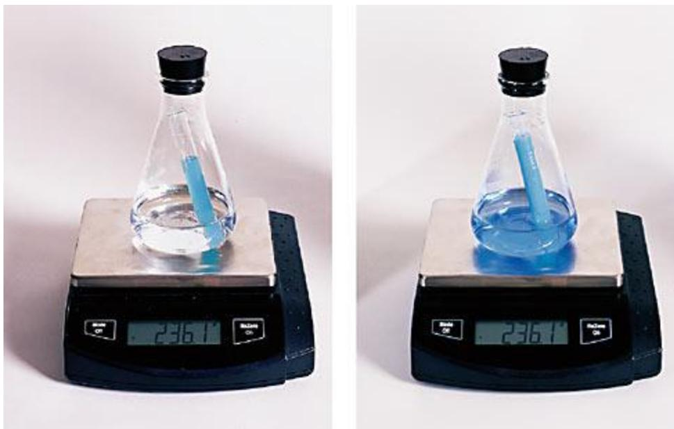
**Figure 8** The total mass before the chemical change is always the same as the total mass after the change.
