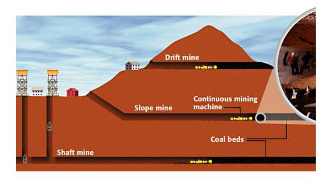
**Figure 3** In subsurface mining, machines such as continuous mining machines (inset) are used to extract ore and load it onto conveyors or shuttle cars.
