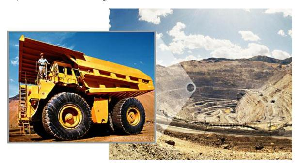
**Figure 2** In open-pit mines, the ore is mined downward in layers. The stair-step excavation of the walls keeps the sides of the mine from collapsing. Giant haul trucks (inset) are used to transport ore from the mine.
