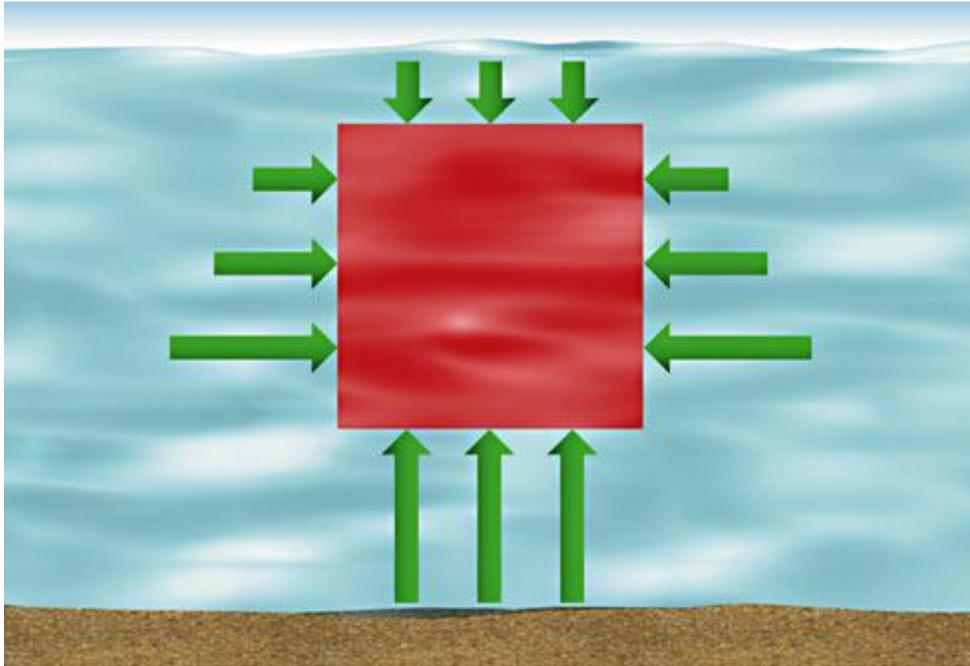
**Figure 1** There is more pressure at the bottom of an object because pressure increases with depth. This difference in pressure results in an upward buoyant force on the object.
