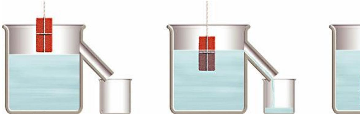
**Figure 2** As a block is lowered into a container of water, the block displaces a certain volume of water. Then, this same volume of water flows into a smaller container. **What does the weight of displaced water in the smaller container represent?**
