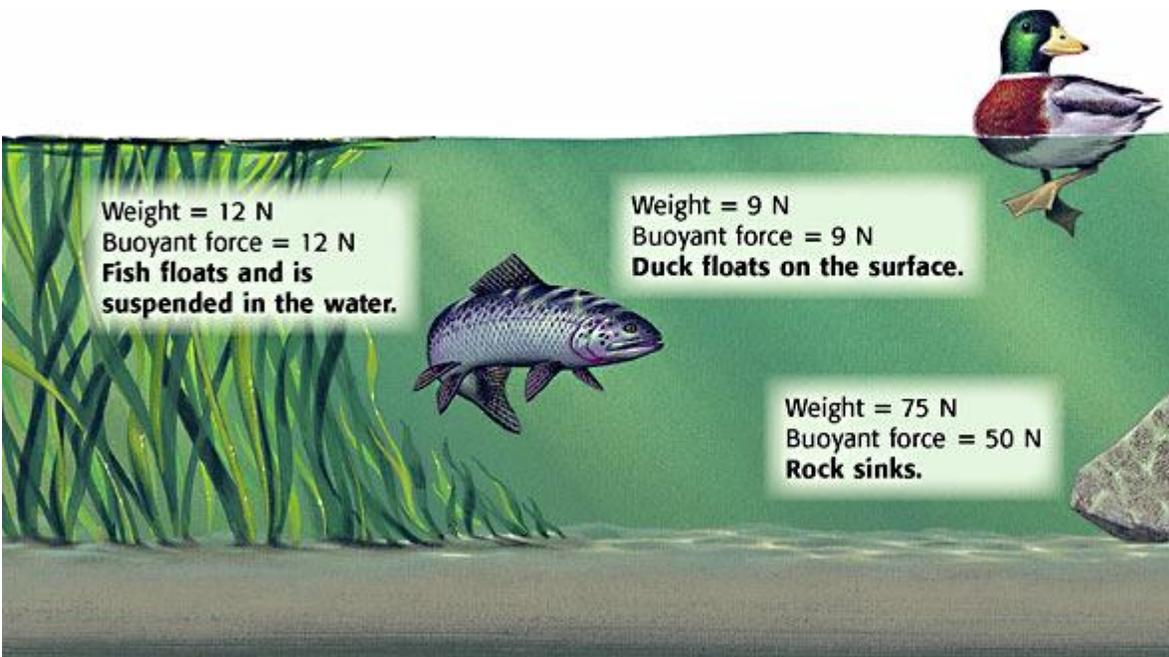
**Figure 3** Will an object sink or float? The answer depends on the amount of buoyant force in relation to the object's weight.
