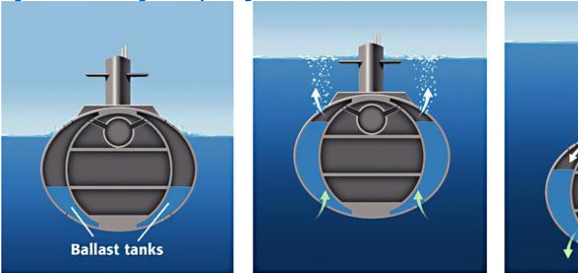
When a submarine is floating on the ocean's surface, its ballast tanks are filled mostly with air.
