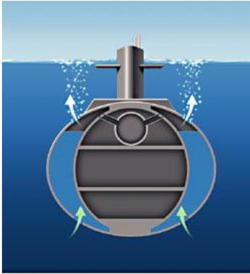
Submarines adjust their overall density by using ballast tanks. This change in density allows them to sink or float.
