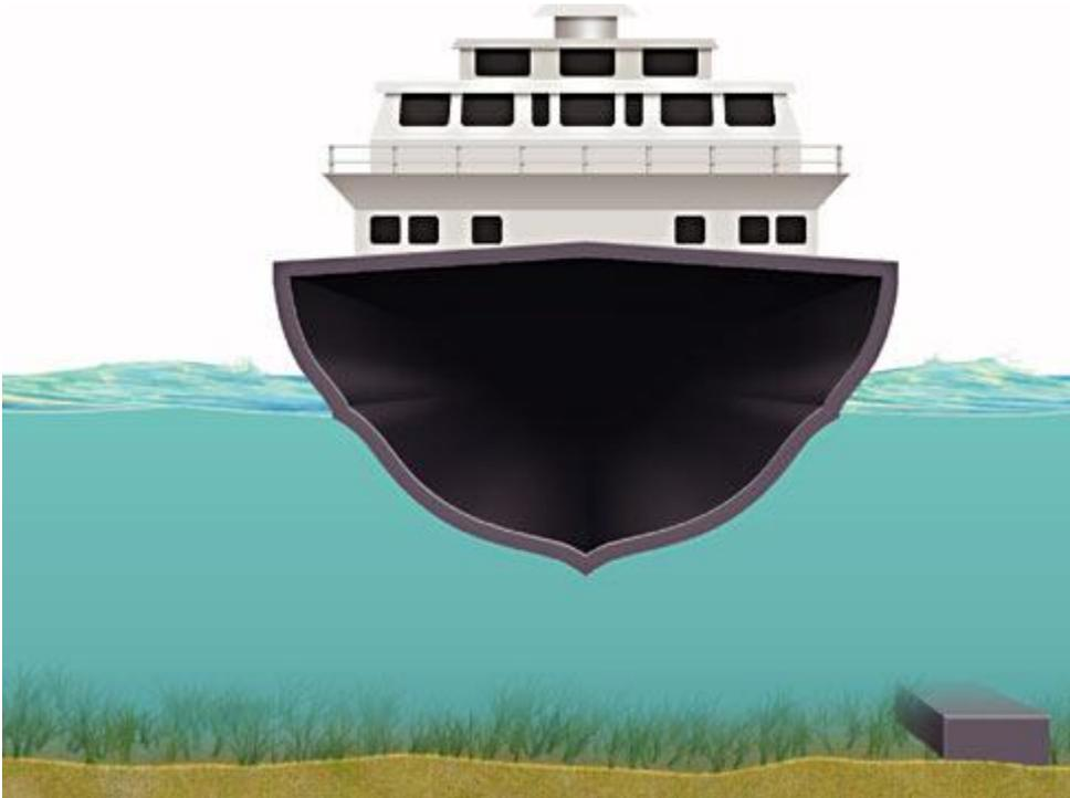
**Figure 5** A block of steel is denser than water, so the block sinks. But shaping that block of steel into a hollow form results in less overall density. So, the ship floats.
