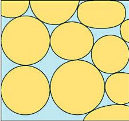
In sandy soils that lie beneath the water table, sand grains are normally in contact with one another.
