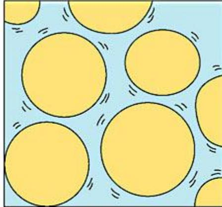
An earthquake causes sand grains to lose contact with one another and to vibrate more violently.
