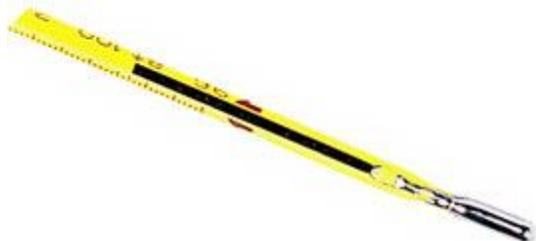
**Mercury** is used in thermometers. Unlike the other transition metals, mercury is liquid at room temperature.
