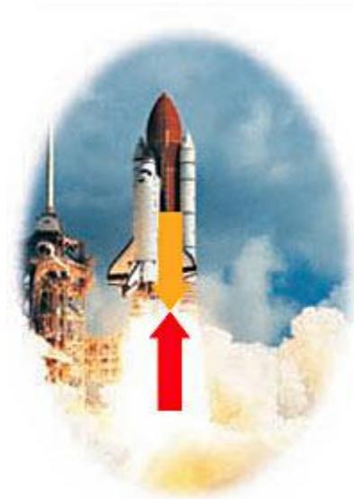
The space shuttle's thrusters push the exhaust gases downward as the gases push the shuttle upward with an equal force.
