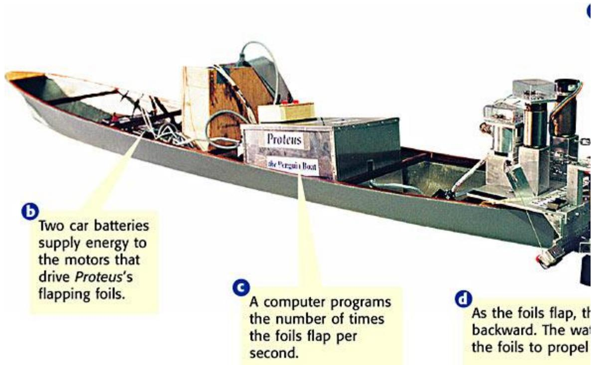
**Figure 4** *Proteus*, a 3.4 m long and 50 cm wide specially built boat model, was used to test the “flippers” hypothesis.
