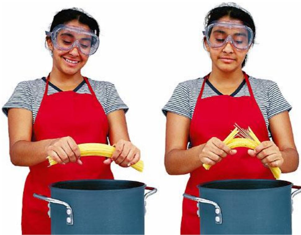
**Figure 1** When a small amount of stress is placed on uncooked spaghetti, the spaghetti bends. Additional stress causes the spaghetti to break.
