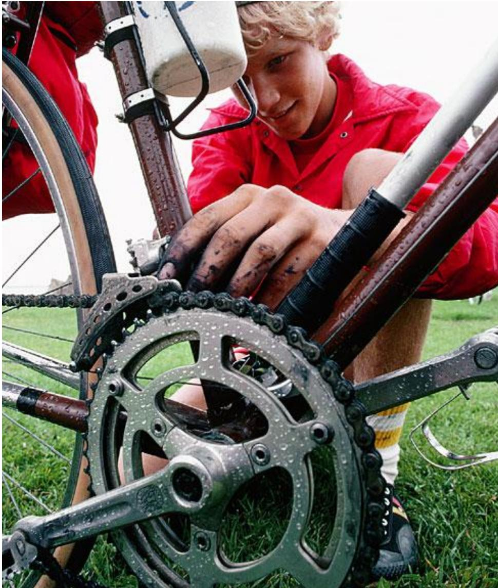
**Figure 5** When you work on a bicycle, watch out for the chain! You may get dirty from the grease or oil that keeps the chain moving freely. Without this lubricant, friction between the sections of the chain makes riding difficult.
