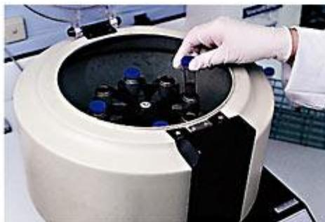
Blood is separated into its parts by a machine called a **centrifuge** (SEN truh FYOO). In the test tube of blood at left, a layer of plasma rests atop a layer of red blood cells. A centrifuge separates mixtures by the densities of the components.
