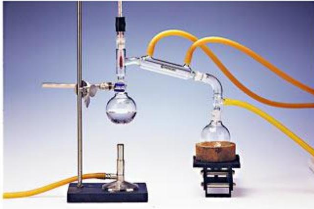
**Distillation** (dis tuh LAY shuhn) is a process that separates a mixture based on the boiling points of the mixture's components. Pure water (flask on the right) is being distilled from salt water (flask on the left). Also, distillation is used to separate crude oil into components, such as gasoline.
